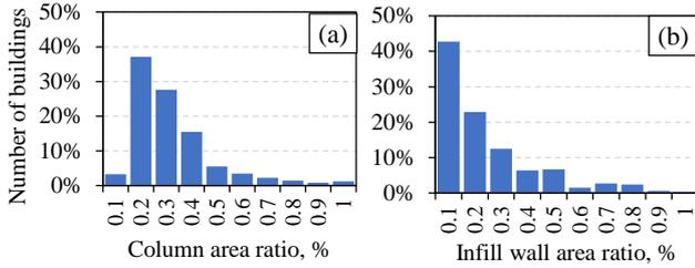
Figure 3: Distribution:(a) column area ratio, (b) infill wall area ratio
