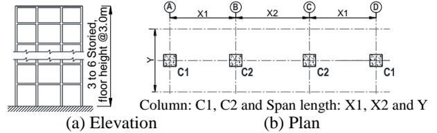
Figure 5: Typical designed RC frame
