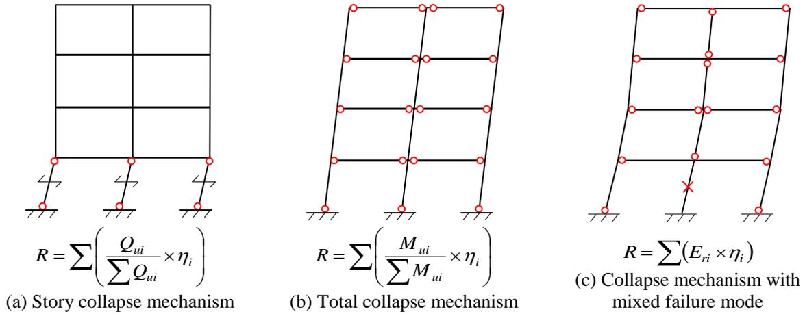
**Figure 1.1.** General concept of  $R$ -index and target collapse mechanism
