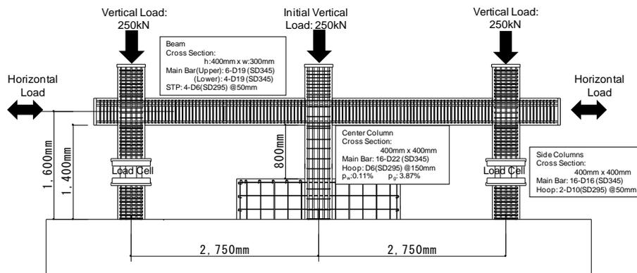
Figure 5.1. Side view of single-story and two-bay frame specimen
