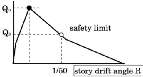
Figure 3.1. Assumed shear capacity for brittle members
