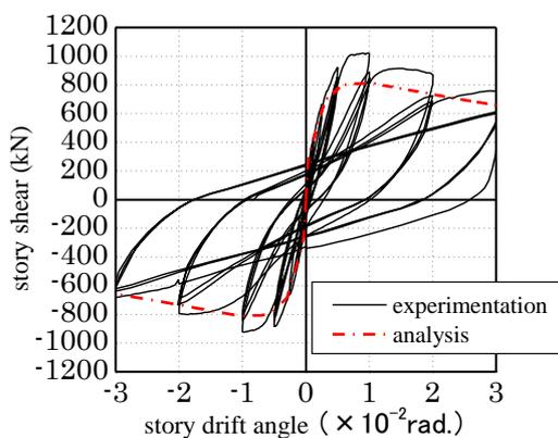
Figure 5.2. Story shear – drift angle of frame specimen
