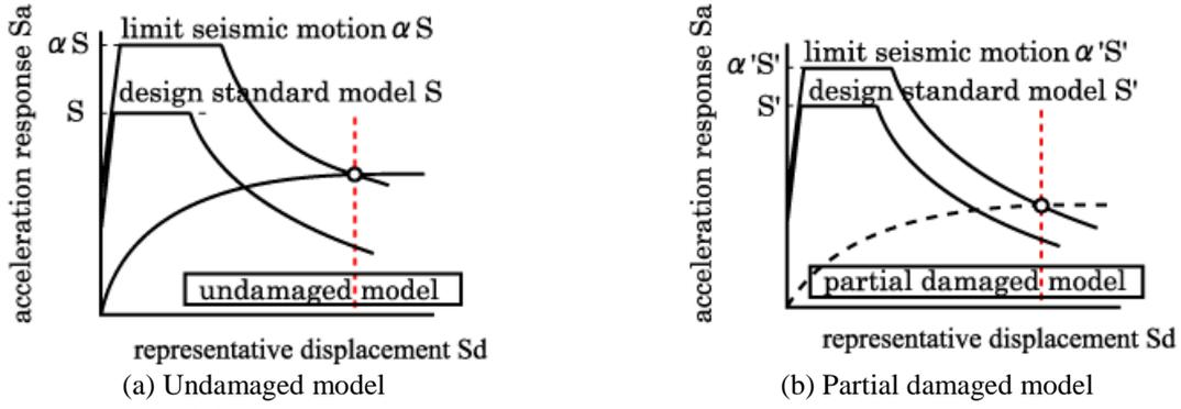
**Figure 2.2.** Seismic capacity index  $\alpha$  for undamaged and partial damaged models
