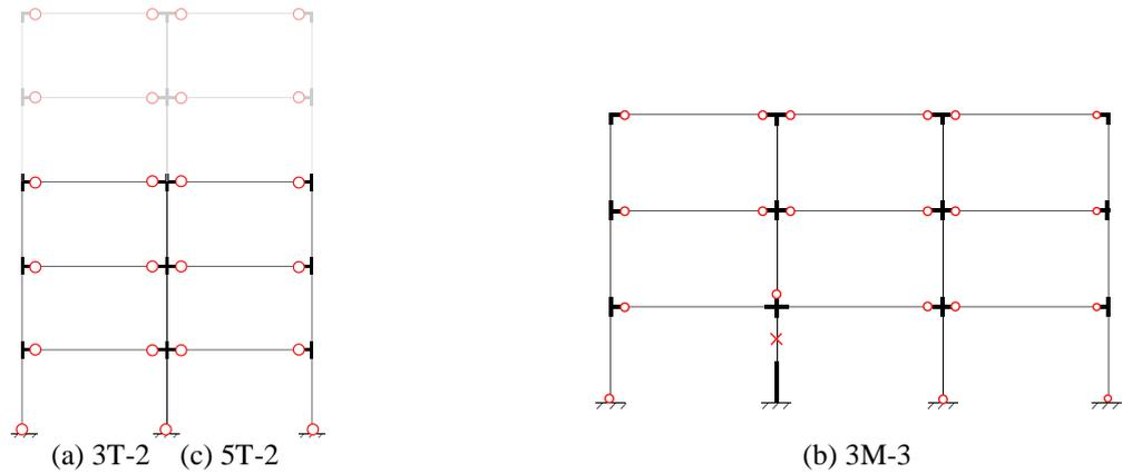
T: beam yielding total collapse mechanism
