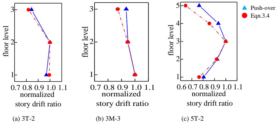
Figure 3.5. Distribution of story drift of undamaged models
