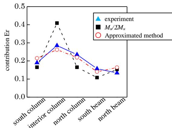
Figure 5.3. Comparison of contribution factor,  $E_r$ , in experiment with calculation
