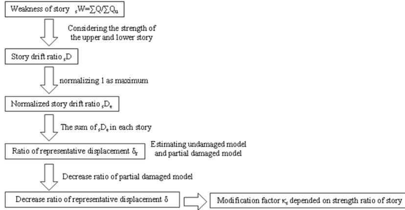
Figure 3.3. Flow of evaluation of modification factor  $\kappa_b$
