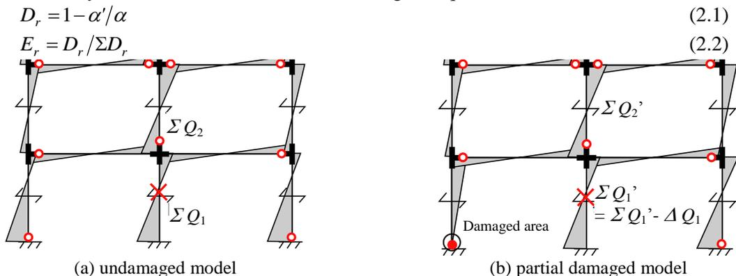
**Figure 2.1.** Story shear capacity at ultimate limit state
