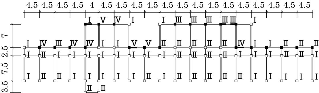
Figure 6.1. Damage distribution in the first story of the damaged RC school building
